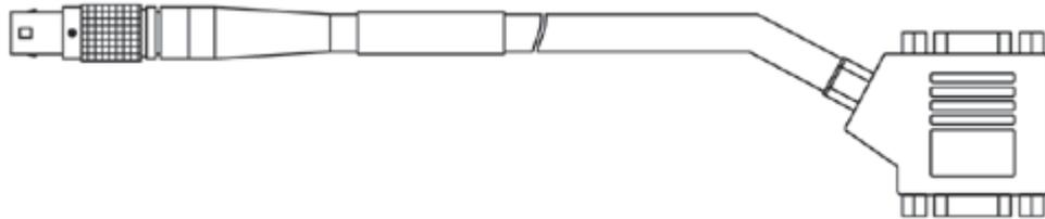
CAN 인터페이스 Y-Cable, Lemo 1B FGC - Lemo 0S PCA - LEMO 0S FFA (8mc-2fc+2mc), 2 m      2.00 m      K107      F-00K-001-272
