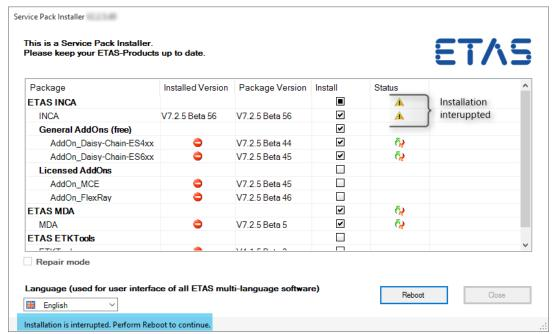
Service Pack installer is interrupted to perform the reboot, indicated in the status bar and icon. After pressing reboot, the system will reboot after a short delay and SPI continues installation automatically after reboot is performed.
